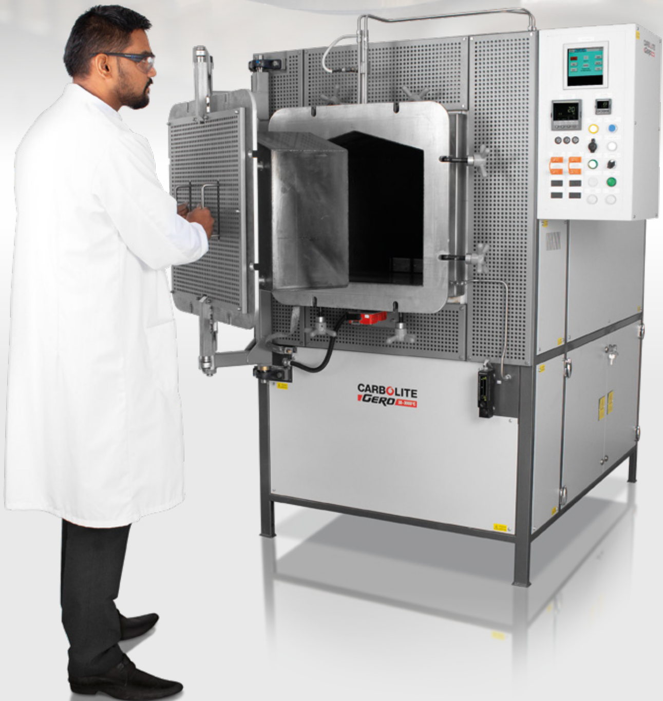
Fig. 1: GPCMA Modified Atmosphere Furnaces for stress relieving of parts manufactured by SLM at temperatures up to 1200°C with a possible oxygen content < 30 ppm.
