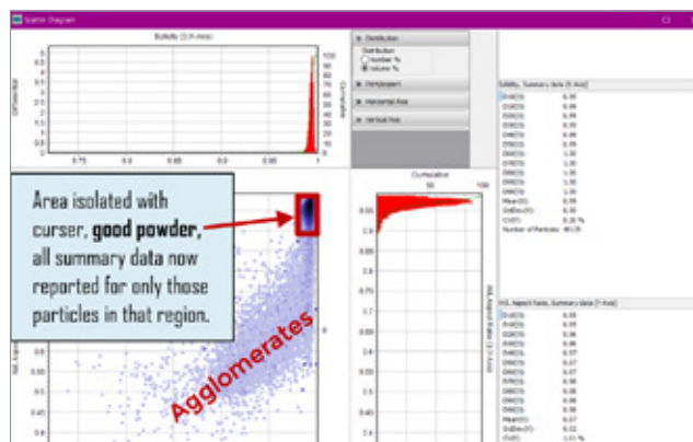
Fig. 6: Analysis of particle shape of 10 different metal powders with Dynamic Image Analysis (CAMSIZER X2). Beside the quantitative results, the recorded images allow an intuitive understanding of morphology and size differences. More spherical particles with higher aspect ratio plot on the right side of the diagram. Detecting the smallest amounts of irregular particles in a large quantity of predominantly spherical particles is a great advantage of DIA.
